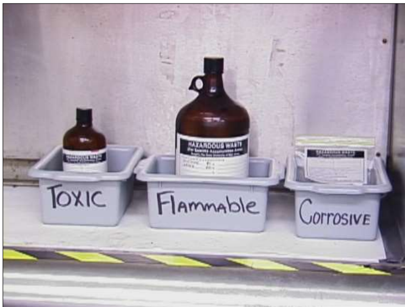
Figure 1. Example of Properly Stored Hazardous Waste in SAA
